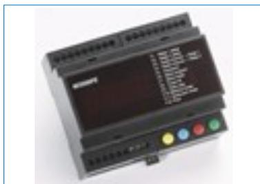
**RFID CARD ACCESS CONTROL:** The M1000 controller is a basic system designed to operate two boom gates. It is a stand alone system and can easily be programed to void cards using the LCD display on the unit.
