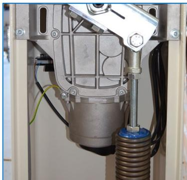
A durable, high quality spring efficiently balances the boom pole. The spring is rated for over 3 million operations.
